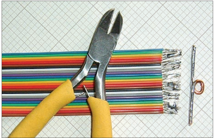
Fig. 1: Carefully pare back the insulation of all the wires by about 10-12mm and tin the ends.
