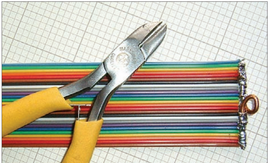
Fig. 2: Then solder the shaped 'end-piece' (made from heavier plain copper wire) in place.
