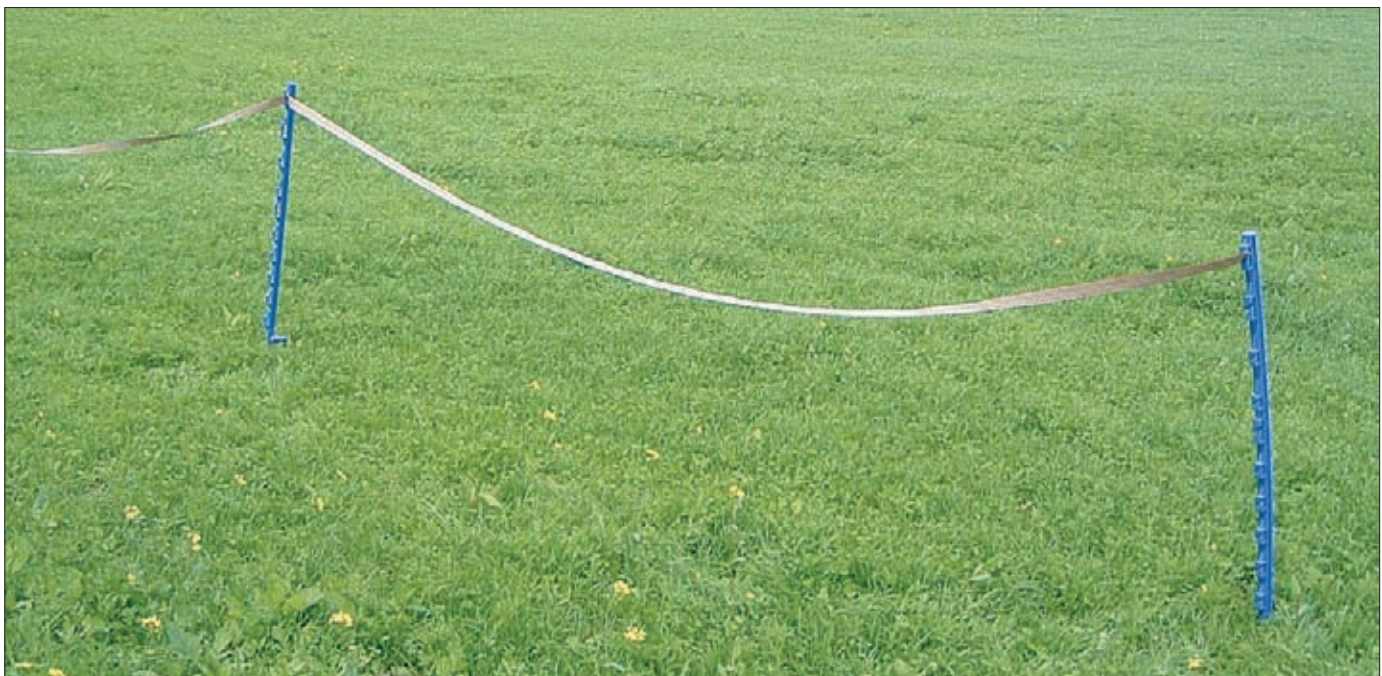
One end of Roy's 'Rainbow' antenna set out as an NVIS antenna.
