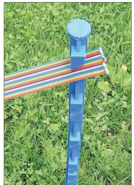
Fig. 4: The end of the NVIS installation, can be held in the 'clamps' of an insulated pole designed for electric fences.
